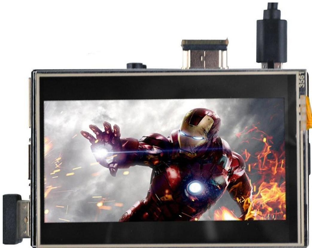
**Step 11:** If you can't see full screen, you can adjust resolution setting, i.e. set to 810 x 540. Please change the config.txt file in SD card, find the line hdmi-cvt and change the resolution in this line. After changing config.txt, save and restart Pi.
