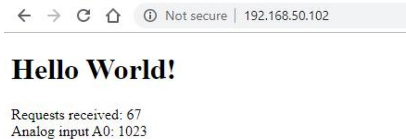
Above result also shows the A0 pin input voltage through `analogRead(0)` function in line 94. `analogRead()` can read the input 0-5V voltage and return a value between 0 to 1023 standing for the voltage. We have connected A0 to 5V, so above Analog input A0: shows 1023.
