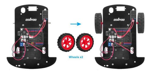
Now hardware installation is almost done. Before we install the battery into the box, we need to upload the sample code into OSOYOO UNO for Arduino first.
