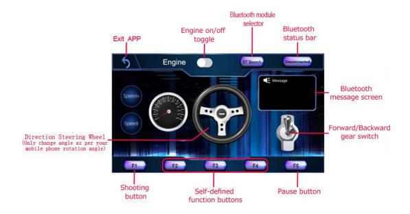
BT Search button: When click this button, you will see a Bluetooth device list which has been paired with your APP. Select HC-02 device to connect the car. Once HC-02 is connected, Bluetooth Status will
