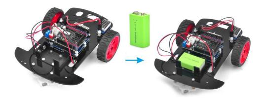
Put the car on the ground, turn on the switch of OSOYOO Motor Shield, the car should go forward, then go backward, then left turn, then right turn, then stop.
