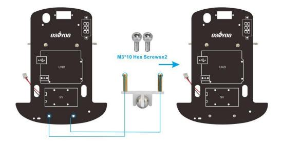
**Step 5.** Install OSOYOO UNO Board on the chassis with M3 plastic screws, pillars and nuts:
