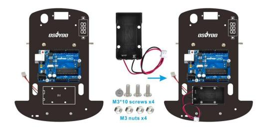
Step 7. Plug the OSOYOO Motor Shield Board in OSOYOO UNO board:
