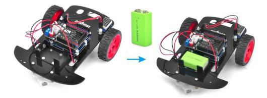
Put the car on the ground, turn on the switch of OSOYOO Motor Shield V1.0, the car should go forward, then go backward, then left turn, then right turn, then stop.
