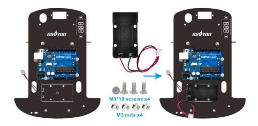
Step 7. Plug the OSOYOO Motor Shield V1.0 Board in OSOYOO UNO board:
