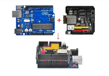
Make sure jumper cap connected E\_TX to D4 and E\_RX to D5.
