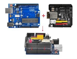
Make sure jumper cap connected E\_TX to D4 and E\_RX to D5.
