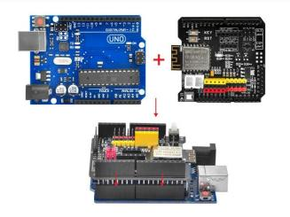
Make sure jumper cap connected E\_TX to D4 and E\_RX to D5.
