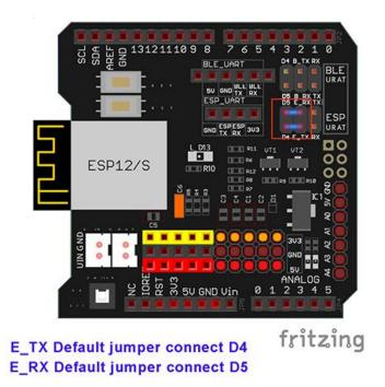
Then connect the LED long pin to D13 in Wifi shield through a 200 ohm resistor, LED short pin to GND, circuit is as below:
