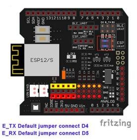
Hardware A) Arduino UNO Board+ESP8266 WIFI shield connects to PIR motion sensor
