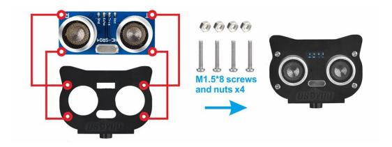
**Step 4:** Install mount holder for Ultrasonic Module on servo motor with M2\*4 Self Tapping screw
