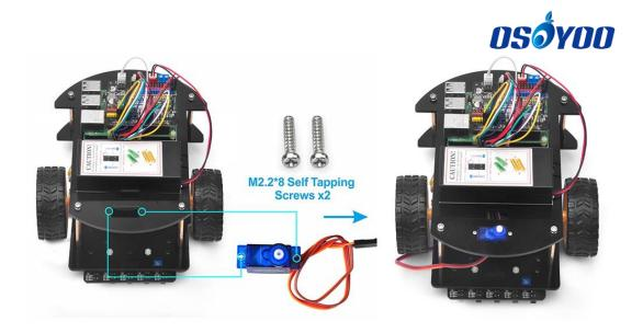
**Step 3**: Choose slotted bracket in servo motor to cross Camera holder from top to bottom and fix blade with M1.5\*6 Self Tapping Screws
