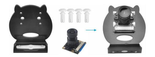
Step 5: Install Camera holder on servo motor with 1pc M2\*4 Self Tapping Screws
