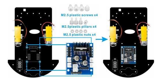
5) Install voltage meter on lower car chassis with 2pcs M2.5 plastic screws, plastic pillars and plastic nuts.
