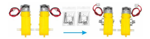
3) Install 2 motors on lower car chassis with screw M3\*10. (Screws in metal motor holder package. Please add M3 washers between screws and chassis if the screws come off easily.)
