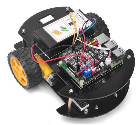
**Step 2:** Install tracking sensor modules under lower car chassis with 2pcs M2.5 plastic screws, M2.5 plastic pillars and M2.5 plastic nuts.
