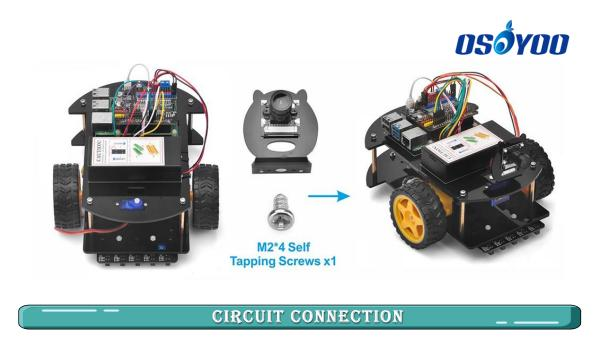
Step 1) Servo Must be installed and connected PCA9685 PWM 15 port
