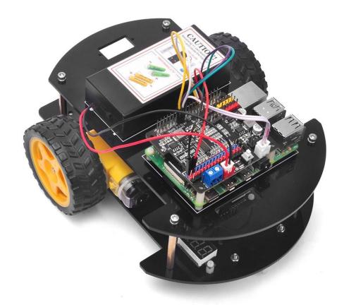
**Step 2**: Install servo motor at the front of upper car chassis with 2pcs M2.2\*8 Self Tapping Screws
