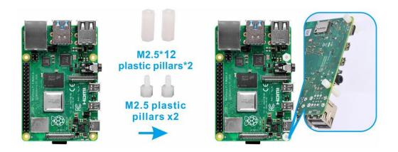
12) Install 2pcs M2.5 plastic screws under the chassis and 2pcs M2.5 plastic screws on Raspberry Pi
