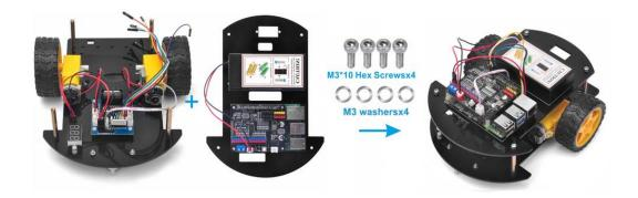
Step 6: Please install your 18650 batteries in battery box for 18650 as per following instruction (Note:Check the box instruction and make sure polar direction is correct, otherwise it can destroy your device and cause fire hazard.)
