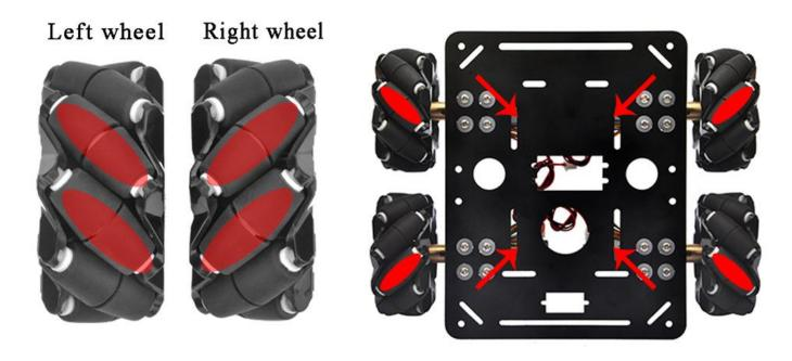
Different rotation combination of 4 wheels will result in different car movement directions. Following pictures shows how they works.
