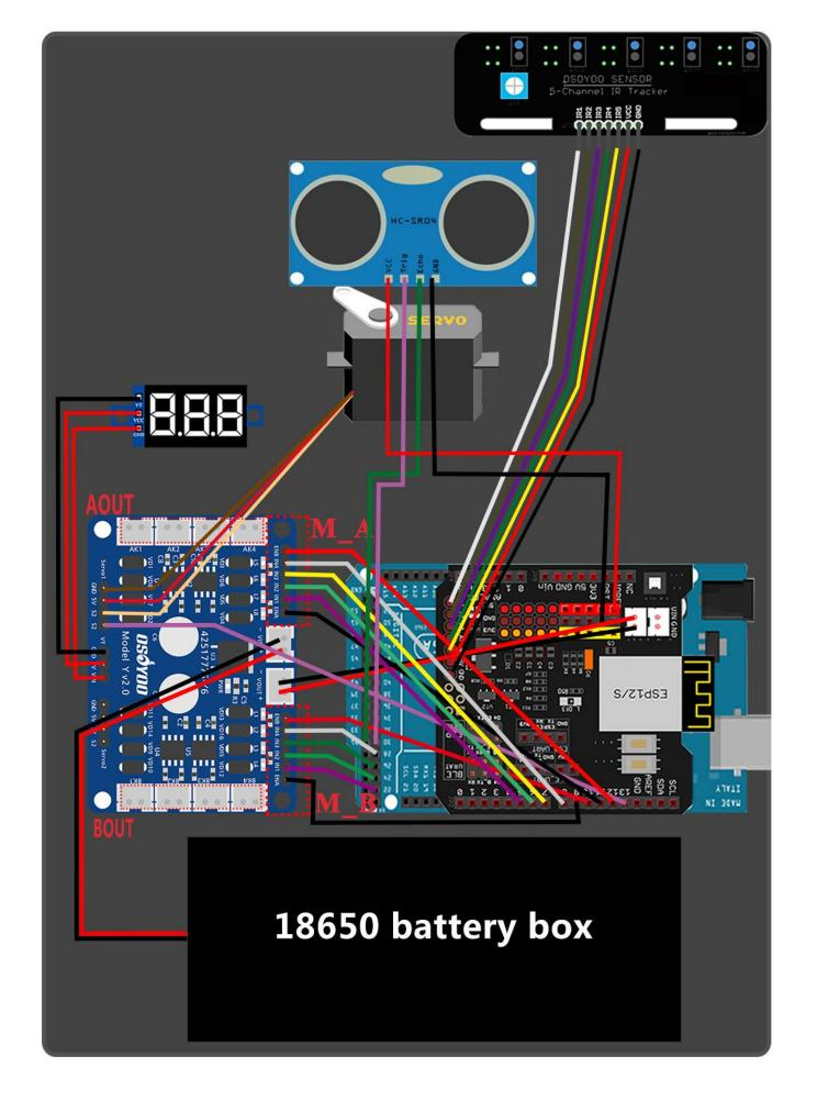
STEP11. Connect 4 motors to model Y driver board as per the following pictures.
