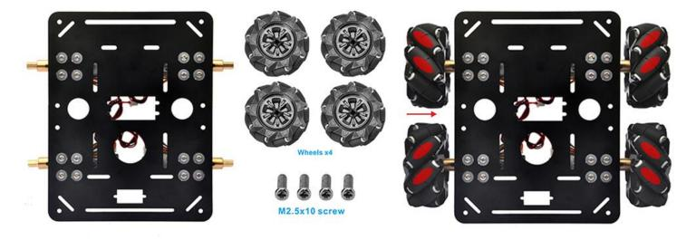
The Mecanum wheel has some sub-wheels on the main wheel. The four Mecanum wheels have
