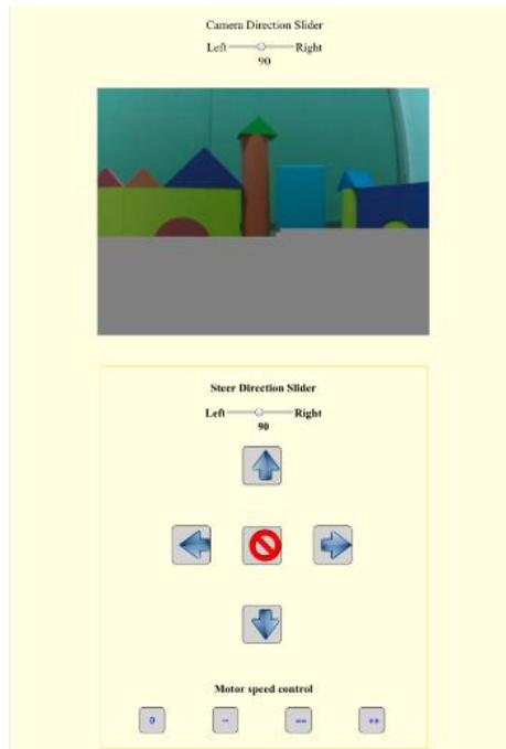
The arrows buttons are direction control keys, red circle button in the middle is the STOP key. There are four speed control buttons in the bottom:
