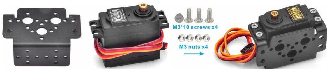
7. Use M3\*10 screws cross servo motor holder with servo motor, lower chassis and nut to fix servo motor on lower chassis as follow:
