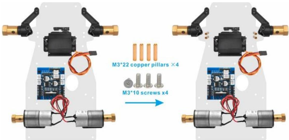
15. Install triangular Acrylic sheets on the M3\*22 copper pillars and fix these with M2.2\*8 self-tapping screws and M3\*10 screws as follow:
