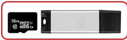
Insert the SD card into SD card reader, then plug card into computer USB port.
