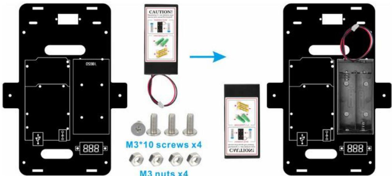
Step8. Attach the voltage meter to the designated markings on the lower chassis using two M3 plastic screws, two M3 plastic pillars, and two M3 plastic nuts. (It is recommended to install the plastic pillar with the male end facing upward.)
