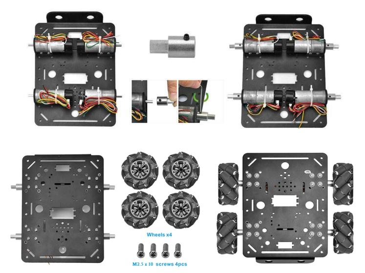
The Mecanum wheel has some sub-wheels on the main wheel. The four Mecanum wheels have two types by the sub-wheel directions. Check the type A wheel and type Wheel by following **picture left side**. You must 100% sure that correct type of wheel is installed into correct position as per **picture right side**, the rolling direction of each wheel will determine the whole car moving directions showed in the picture.
