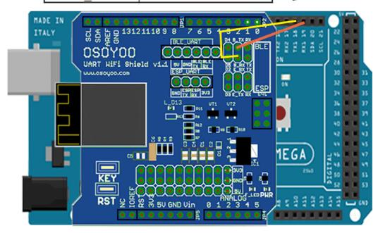
$\it STEP2:$ Bluetooth Module should be inserted into bluetooth 6-pin slot in OSOYOO Wifi Board
