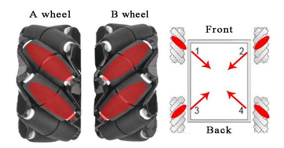
Different rotation combination of 4 wheels will result in different car movement directions. Following pictures shows how they works.
