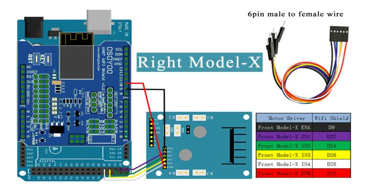
Note: wire(purple wire) is connected to D22 which is located on the SECOND female hole from right in following picture 10. Many people treat the first hole as D22. THIS IS WRONG.
