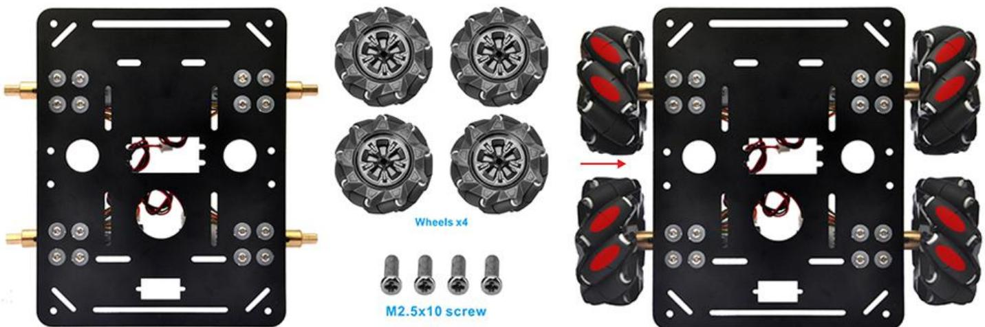
The Mecanum wheel has some sub-wheels on the main wheel. The four Mecanum
