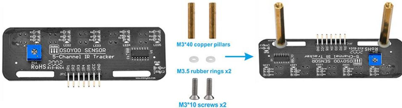
STEP2. We have added a 5-Point tracking sensor module to the car chassis with M3 nuts in lesson1 as following pictures.
